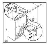
Insert the two fixing brackets into the slots provided in the top front part of the dishwasher, as shown in the figure.
